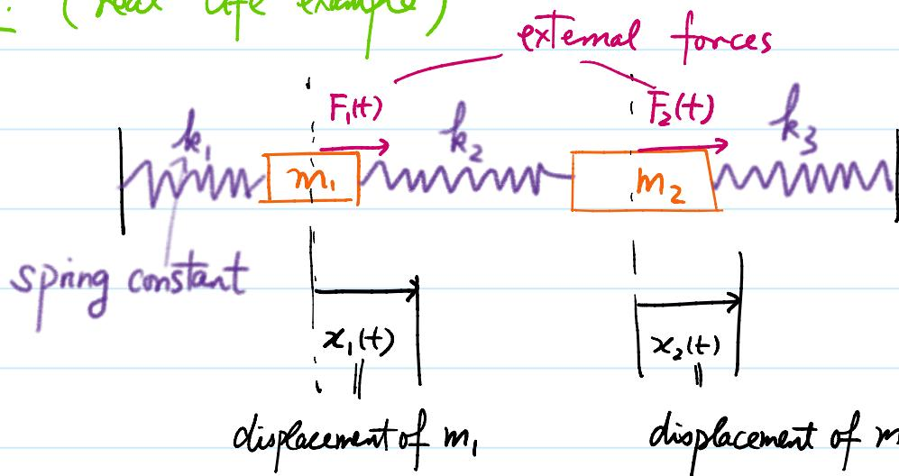
$\bar{F} = ma$  Equation for  $m_1$ :  $m_1 \frac{d^2x_1}{dt^2} = -k_2(x_2 - x_1) - k_1 x_1 + F_1(t)$
